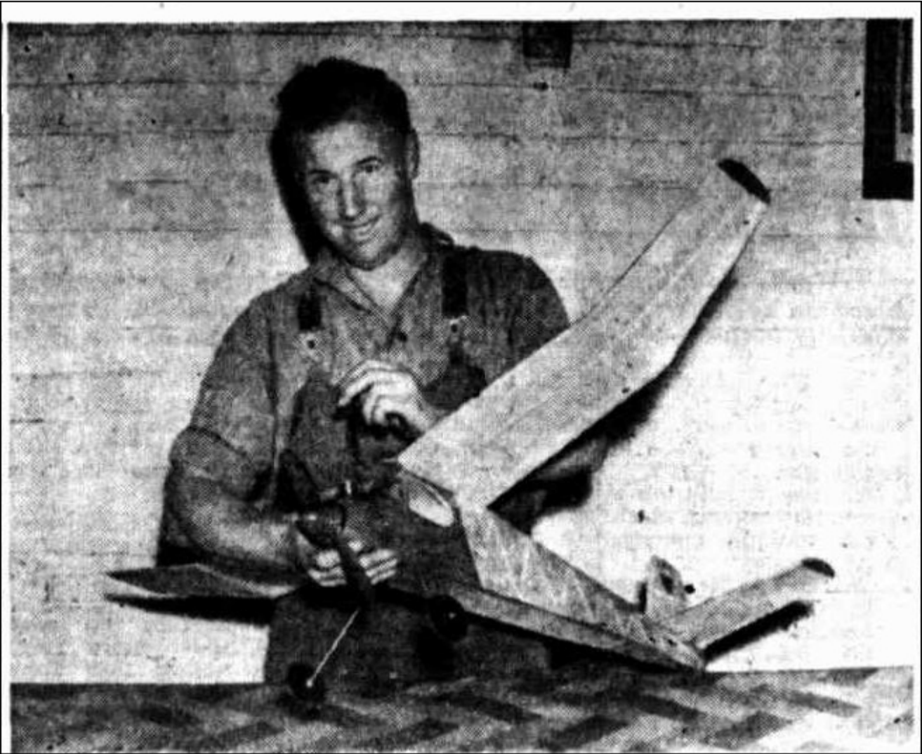
Mr. Norm Lancaster with one of the model aeroplanes which he builds himself. This is a free-flight model with a wing span of four feet, and Norm says it has an "E.D. 2cc competition special diesel" engine.
